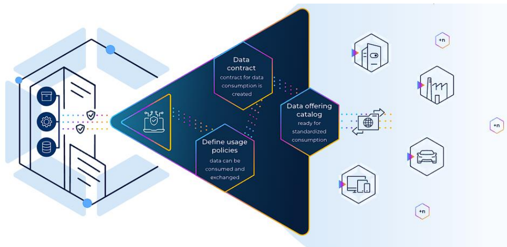
Figure 27: Premises – Connector – Data space, the three key framework components of the NIKH platform
