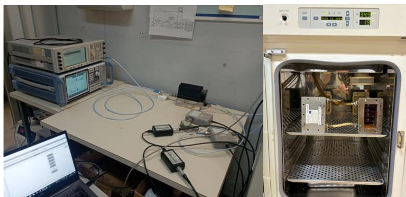
Figure 3: Configuration and components of the setup employed for simultaneous exposures of four samples to 1950 MHz (LTE signal) and 2450 MHz (Wi-Fi) RF-EMF.
