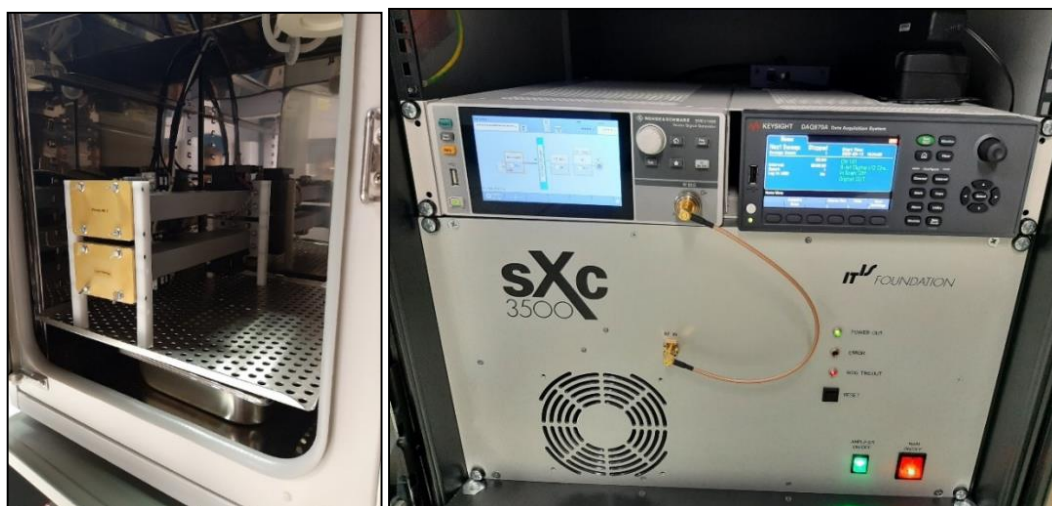
Figure 7: Waveguide-based setup for exposure to a 3.5 GHz, 5G signal electromagnetic field. The waveguides inside the incubator (left) and the signal tower, including the vector signal generator and the amplifier (right).
