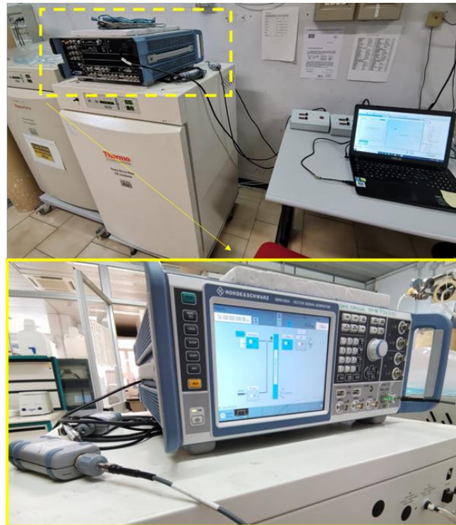
Figure 1. Exposure system setup. The signal is sent to the RC placed inside a cell culture incubator while a second RC, placed inside another cell culture incubator, is used for sham exposure. Each chamber is equipped with two stirrers at independently controlled speed and hosts a sample holder to allow reproducible positioning of the cell culture dishes.
