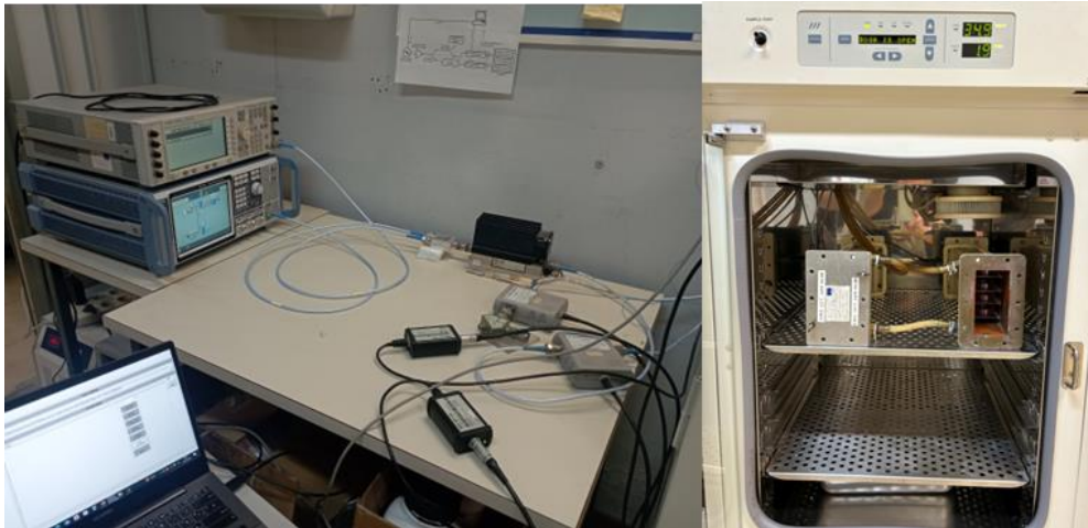
Figure 13: Configuration and components of the setup employed for simultaneous exposures of four samples to 1950 and 2450 MHz RF-EMF.
