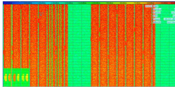
Figure 15: Full-loaded 5G frame; on the left bottom 6 SSBs are visible; the void area in the centre and at the end of the frame are the sections of the frame reserved for uplink data, almost all the remaining area is filled by PDSCH REs (users data).
