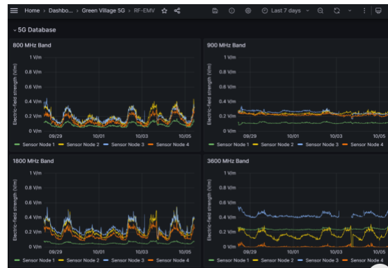
Figure 49: Dashboard developed in Grafana presenting the output of the sensor installed at the Green Village, showing the diurnal rhythm of the electric field strength at that location.
