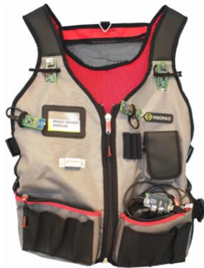
Figure 43: Measurement vest developed by the smart sensor system at The Hague University of Applied Sciences.
