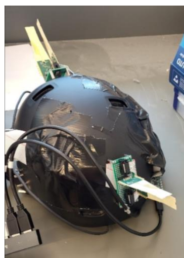
Figure 53: Helm prototype with integrated two (dual polarized) FR2 sensor (prototype zero) realized by the partners and the microcontroller board and logging system developed in the NextGEM and discussed in Section 3.3.1.
