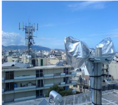
Figure 19: Non-commercial deployment for continuous outdoor EMF monitoring.
