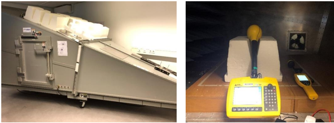
Figure 8: The outside and inside of a GTEM cell. Benchmark equipment (SRM3006) inserted in the GTEM cell [57].
