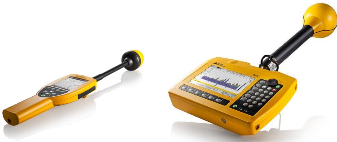
Figure 2: Examples of broadband (left) and frequency-selective (right) EMF measurement equipment.
