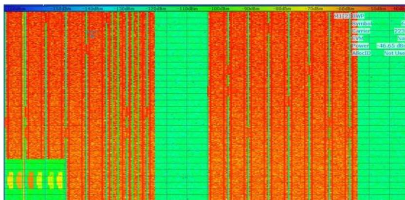
Figure 27: An example of full-loaded 5G frame in downlink connection; horizontal axis: symbols, vertical axis: subcarriers
